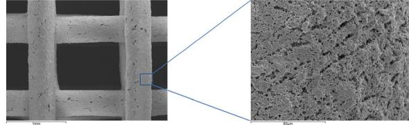
Sepiolite based catalyst supports produced by combined freeze-robocasting technique
