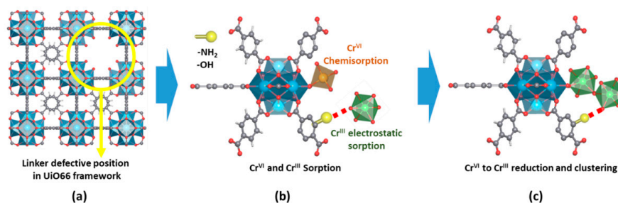
Figure 14. (a) Local structure of a linker defect position in UiO-66. (b) Detail of the possible Cr(VI) and Cr(III) adsorption positions at an under-coordinated defect position and organic linkers of zirconium hexanuclear clusters. (c) Cr(VI) to Cr(III) reduction induced by the presence of electron-donor groups at the organic linkers or photoactivity of the material. Reproduced with permission from reference [65].
