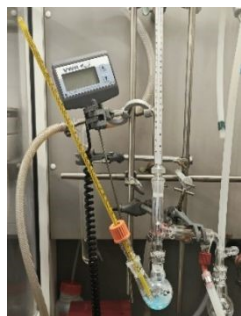
Figure 2. Set-up for the determination of the temperature inside the flask during the dehydration of 1-hexanol.
