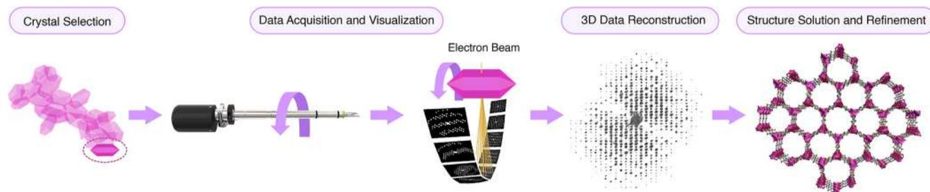
**Figure 1.** Schematic representation of the workflow of a three-dimensional electron diffraction experiment.
